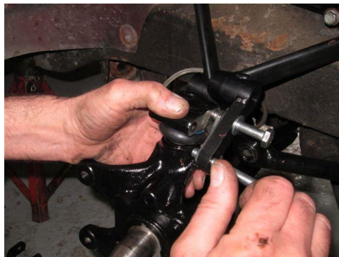
Image 8: Fitting Upper Trunnion
