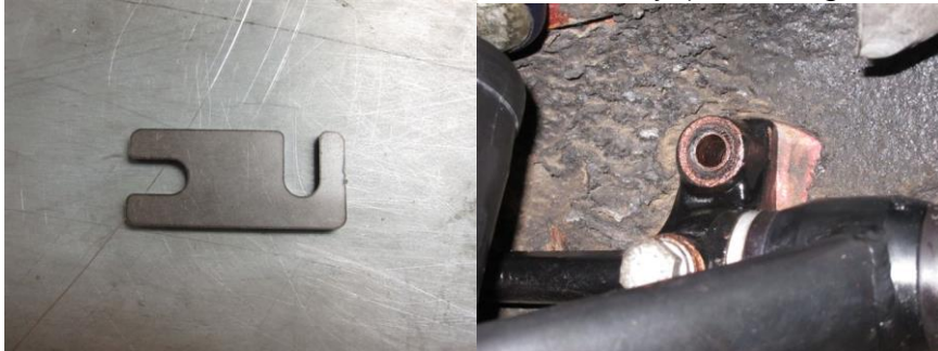
Image 12: Camber Shims, Image 13: Locating Shims behind Pivot
